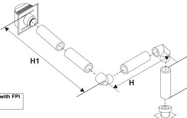
Must Use: 5" x 8" Simpson Direct Vent GS Piping with FPI Increaser Starter Collar (Part #946-605).
